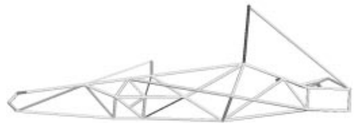
Figure 6. Frame Triangulation (Frame, Side View)
